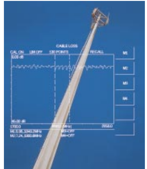
Verify cable insertion loss from ground level.
